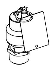
**Technical Requirement:**1. The design, manufacture and inspection of safety valve are based on KS B 6216.
